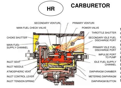
the fuel side of the metering diaphragm. Atmospheric air pressure on the opposite side will force the metering diaphragm upward causing the diaphragm button to contact the inlet control lever and overcome the inlet tension spring pressure, permitting fuel under pressure to force the needle off its seat and enter the metering chamber. The fuel then travels from the metering chamber up through the idle and main fuel supply orifices and channels and out the discharge ports to the engine.
